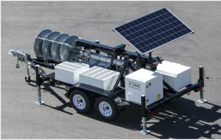
360XT IS AVAILABLE WITH AN OPTIONAL SOLAR PANEL FOR REMOTE CHARGING CAPABILITY
