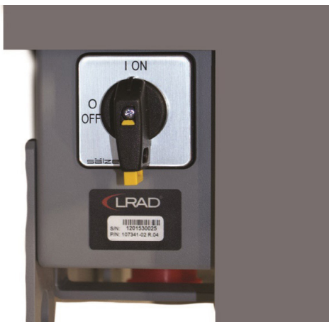
On/Off Switch Directly on Power Supply
